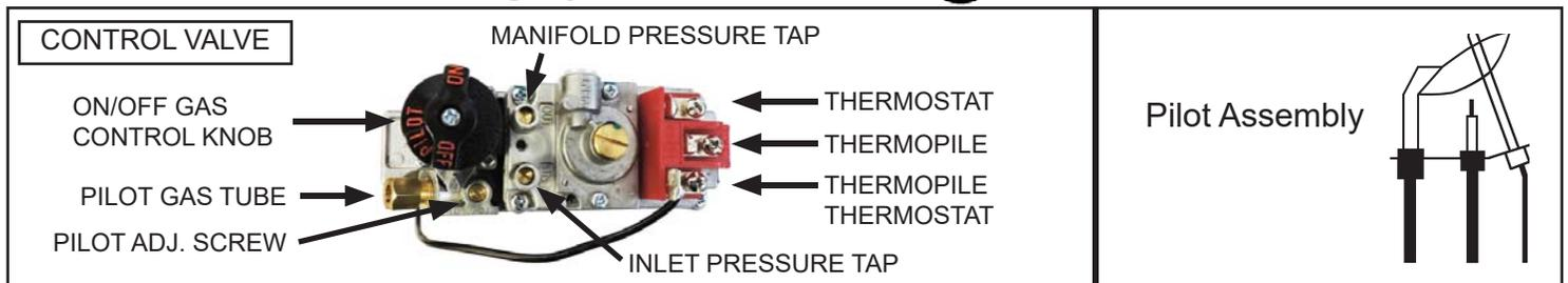
**NOTE:** Knob cannot be turned from "PILOT" to "OFF" unless knob is pushed in slightly. Do not force.
