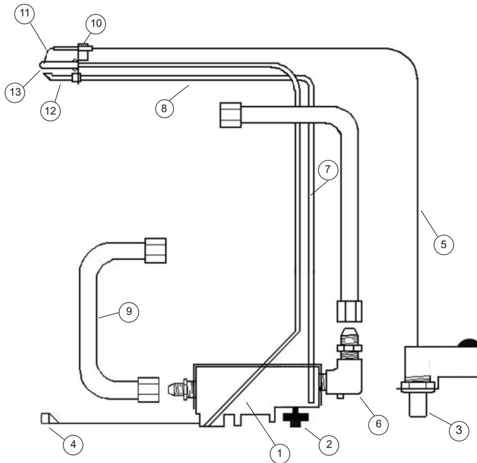
The pilot flame adjustment is labeled on the top of the valve. Locate the pilot adjustment at the upper right hand of the valve near the pilot tube connection.
