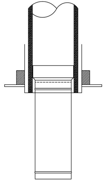
3. Slip the adapter and pipe into the chimney system.
