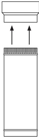
1. Insert a 9" x 24" section of pipe into the smaller end of the 9" to 10" adapter.
