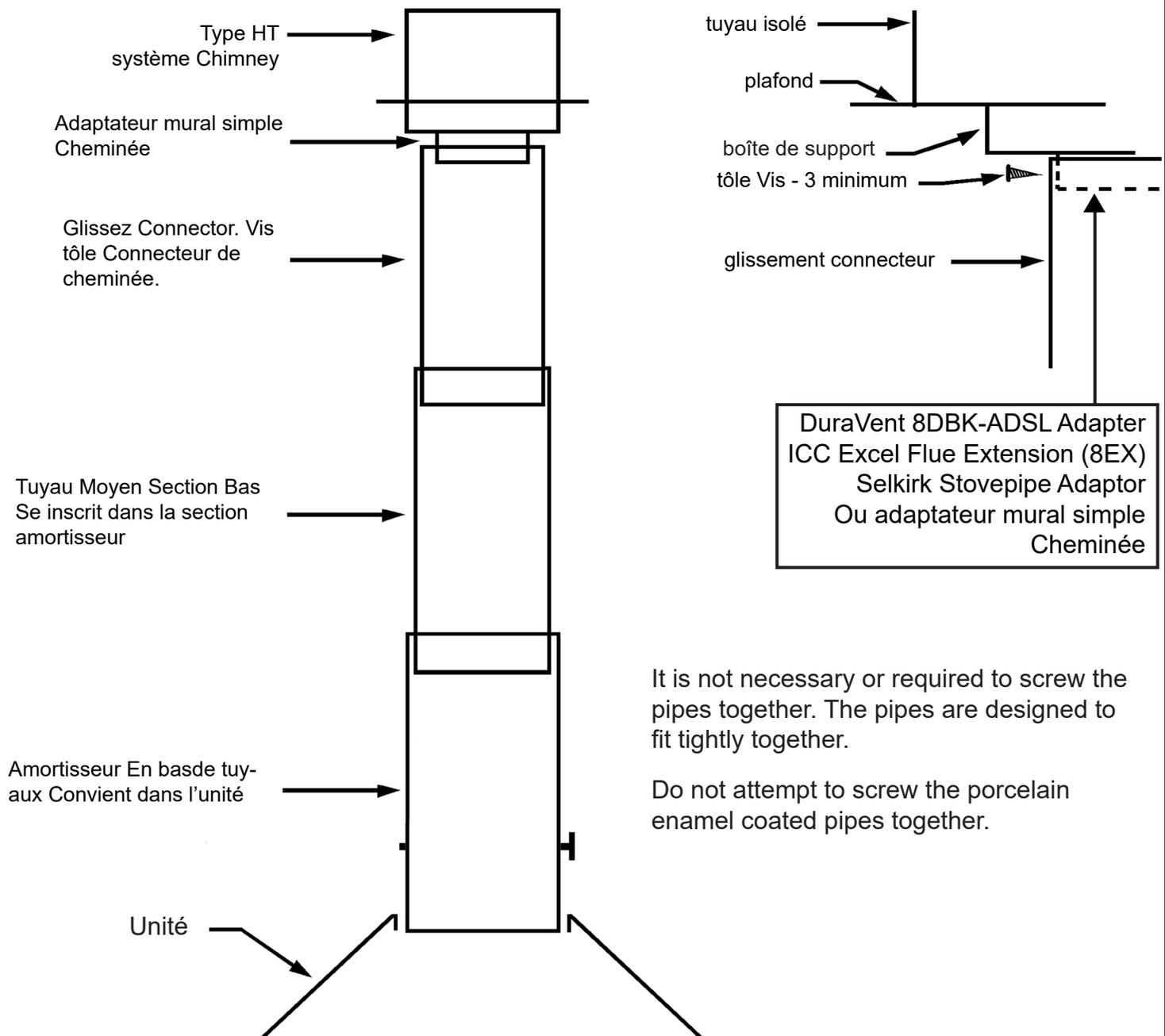
It is not necessary or required to screw the pipes together. The pipes are designed to fit tightly together.
