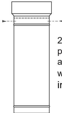
2. Screw the pipe and the adapter together with 3 - #8 x 3/8 inch screws.
